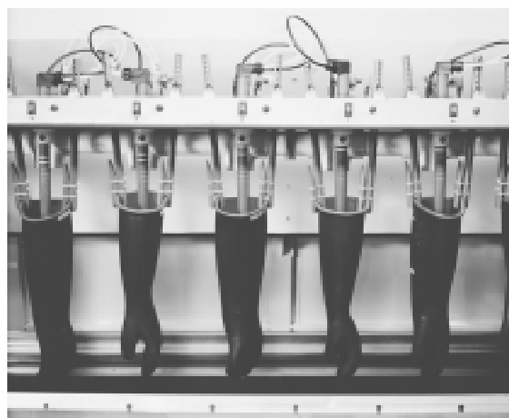
24 position test unit with dual AC & DC power supply
