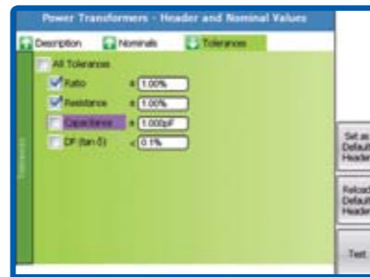
Tolerances window allows setting the tolerances for each of the available tests.
