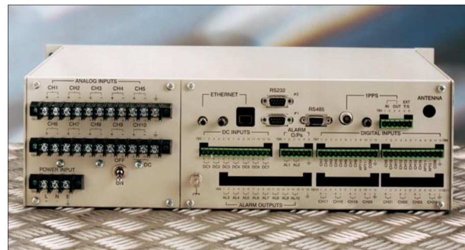
DAU Rear Panel showing Extensive Connections
